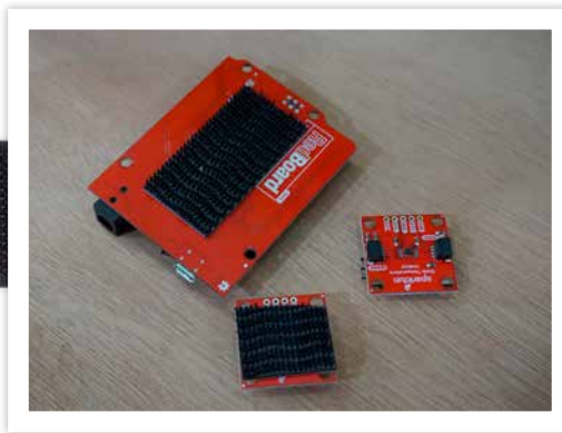
Figure 2: Dual Lock is just the right width for most Qwiic boards, and with the boards being single sided, it sits nice and flat.
