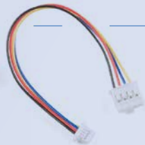
Figure 4: Qwiic adapter for Grove.
